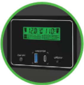
Pantalla LCD, puerto USB de carga TipoC 5V/3A e interruptor selector (UPS-INV)
