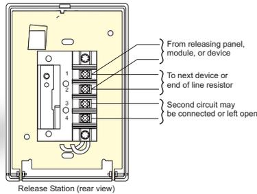
The manual release station is a normally-open, dry contact signal initiating device. The 276A-REL is a single-action station that requires the user to pull the release handle to initiate the release of a fire suppression agent. The 278A-REL (shown) is a double-action station that requires the user to raise the upper door, then pull the release handle to initiate the release.
